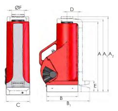
A = JACK WITH PLAIN PISTON A  $_{\mbox{\scriptsize 1}}$  = JACK WITH PLAIN PISTON & LIFTING CLAW & EXTENDED BASE
