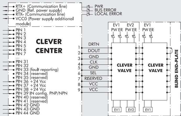
WIRING DIAGRAM FOR THE CLEVER CENTER TERMINAL FOR VALVES AND INPUTS/OUTPUTS
