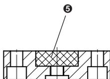
Supplied with two baffle plates. The hard one (white) is premounted.
