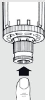
Press the button to drain condensate when the bowl is pressurized.
