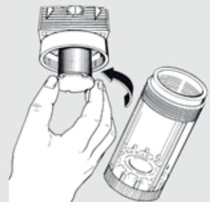
To clean or replace the filter element unscrew the screen of the centrifuge assembly. Use a no. 3 compass spanner to unscrew the bowl.
