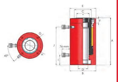
Note: 33 & 61 tonne models feature 2 base mouting holes at 90° from coupler.
