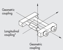
\* Resistance to the reciprocal displacement of two components with a 6 Nm screw torque.
