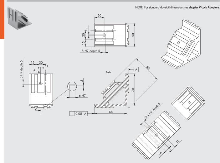
Adaptor suitable for the rotated coupling of two or three V-Lock components, with two supporting surfaces at right angles. The third surface is at 45° angle. All the grooves are parallel.
