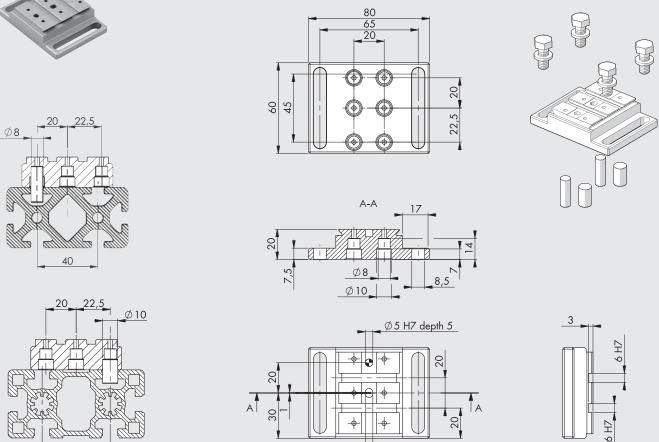
An adaptor for fixing V-Lock components transversally onto extruded profiles, with slots with 40 or 45 mm centre distance or 8 or 10 mm width. If the slots have a 40 mm centre distance, insert two pins in the slots 20 mm from the axis of the adaptor and use them as an alignment reference. If the slots have a 45 mm centre distance, use the 22.5 mm pin slots.
