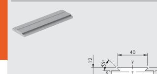
Profile to DIN 17615 (precision profiles). Used for making adaptors.
