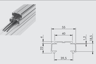
Profile to DIN 17615 (precision profiles). Snap-in profile for the laying of pneumatic hoses and electrical cables.
