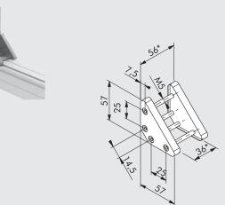
Angled attachment for 90° connections for use in medium load applications.
