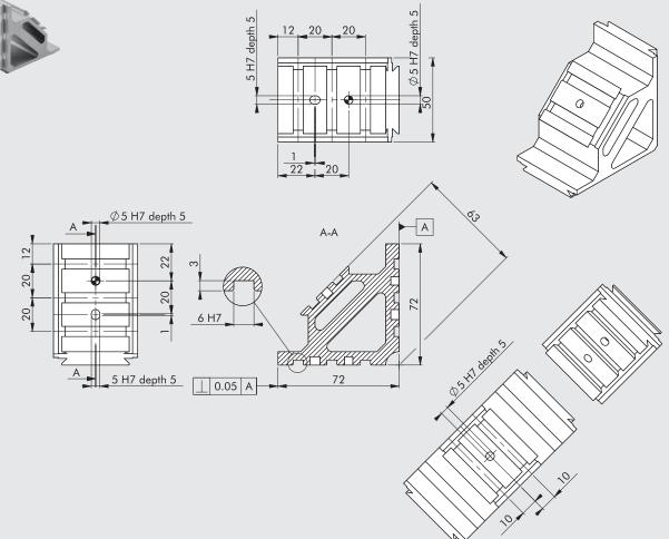
Adaptor suitable for the rotated coupling of two or three V-Lock components, with two right-angle supporting surfaces and parallel grooves. The third surface is at  $45^{\circ}$  angle and the grooves are parallel to those in the other two faces.
