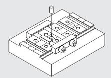
If greater precision is required, one or two Ø 5 pins can be inserted in the slots provided.
