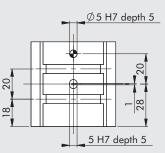
Adaptor suitable for parallel coupling of two V-Lock components, one with at least two grooves and the other with one groove only.
