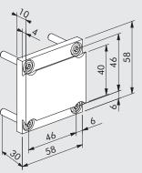
Adapter for front fixing obtained from DIN 17615 profile profiles (precision profiles)
