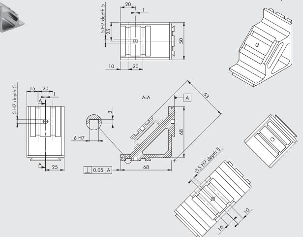
Adaptor suitable for the rotated coupling of two or three V-Lock components, with two right-angled supporting surfaces and grooves at right angles. The third surface is at 45° angle.
