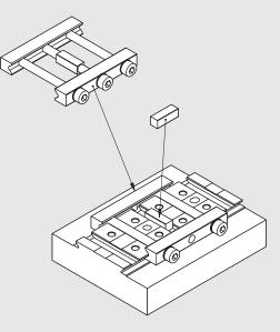
The number and size of fixing elements depend on the specific application. Under operating conditions of high speed, pressure and load, we recommend installing two elements with two screws as spaced as possible from each other.
