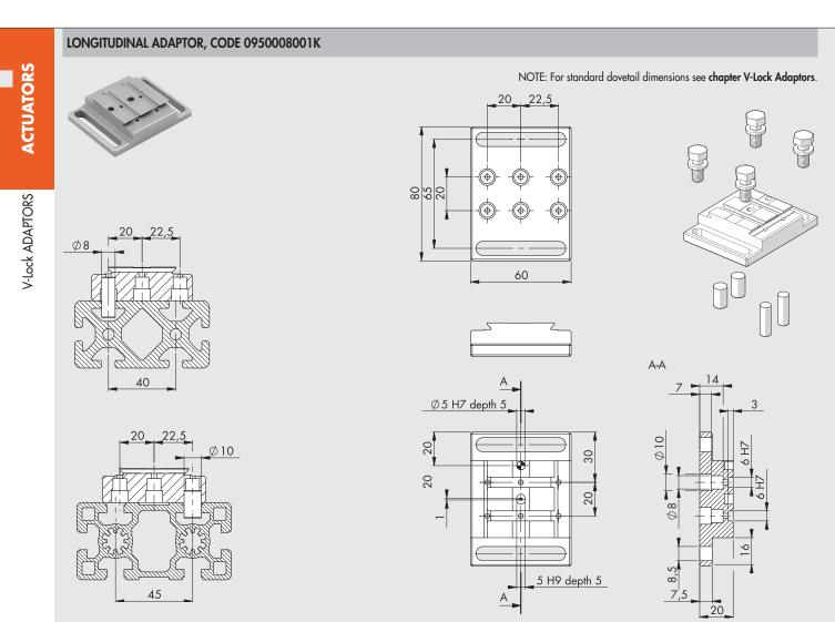
An adaptor for fixing V-Lock components longitudinally onto extruded profiles, with slots with 40 or 45 mm centre distance or 8 or 10 mm width. If the slots have a 40 mm centre distance, insert two pins in the slots 20 mm from the axis of the adaptor and use them as an alignment reference. If the slots have a 45 mm centre distance, use the 22.5 mm pin slots.
