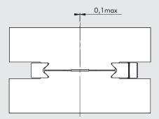
The V-Lock system allows transversal self-centring of the components. If the K blocks are mounted correctly, the alignment error is less than 0.1 mm.
