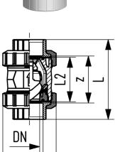
SYGEF Standard Check valve type 561 Without spring With threaded sockets NPT
