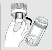
To clean or replace the filter element unscrew the screen of the centrifuge assembly.
